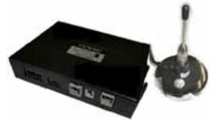
ITS wireless receiver (equipped on vehicle)
