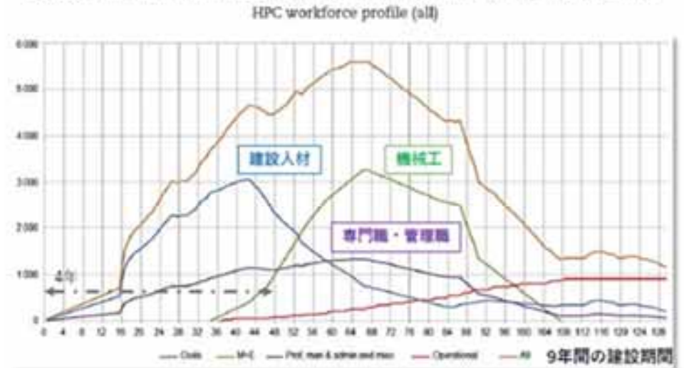
Figure 2.1. FTE labour force requirements at Hinkley Point C (twin EPRs) by quarter
