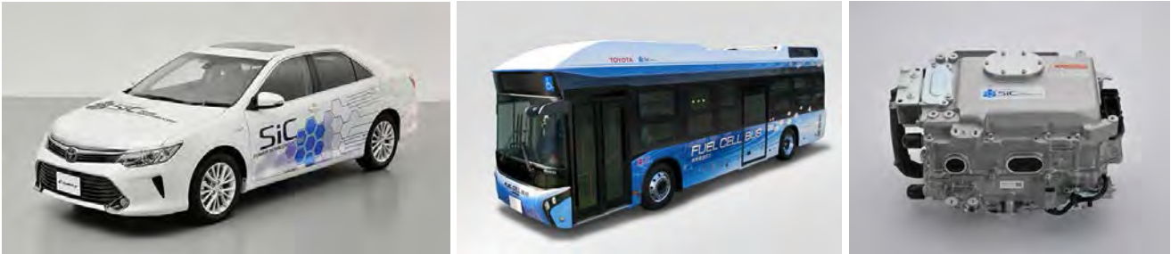
Camry prototype (left) and fuel cell bus (center) featuring SiC power semiconductors; power control unit
