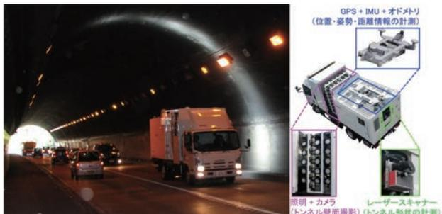
図2 Mobile Imaging technology & Mobile Mapping system (MIMM)
