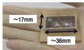
The size of the developed module are less than a quarter of those of the conventional products.
