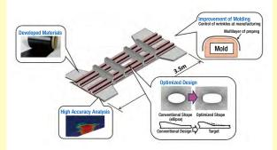
Aerospace grade composites with 50% higher resistance to propagation of internal damage than benchmark materials have been developed along with their optimum structural design and strength characterization method. Subcomponent structures with skin/stringer were fabricated and evaluated under assumed flight loads.
