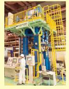
After introducing 1,500 ton forging equipment and constructing the models
