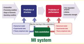
We have developed various kinds of modules for predicting microstructure and performances such as fatigue strength, creep strength, hydrogen embrittlement, brittle fracture, data-driven prediction tools, and the Materials Integration (MI) System, the  $\alpha$ -version based on manual connection of these modules. We aim to automate the system by using information technology and continue to enhance the kinds of modules.
