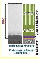
We have developed advanced Environmental **Barrier Coating** (EBC) structure and its manufacturing technologies. We have evaluated the thermal cyclic properties of EBC under simulated atmosphere at 1400°C and then have newly established an evaluation method about the interface toughness for an EBC bounded to a SiC/SiC substrate.
