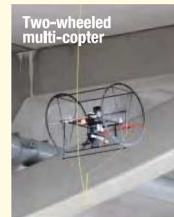
•Bridge Inspection Support Robot System
