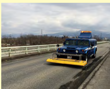
• High Speed Scanning with 3D Radar
