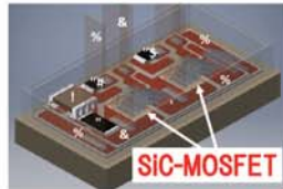
The size of the developed module are less than a quarter of those of the conventional products.
