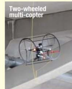
•Bridge Inspection Support Robot System
