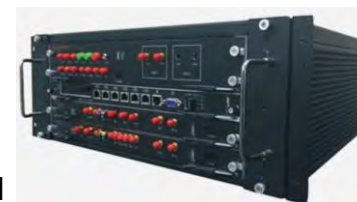
GHz quantum key distribution terminal
