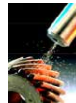
Strengthen materials by iron ball
