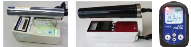
NaI Scintillation Survey Meter(Example)
