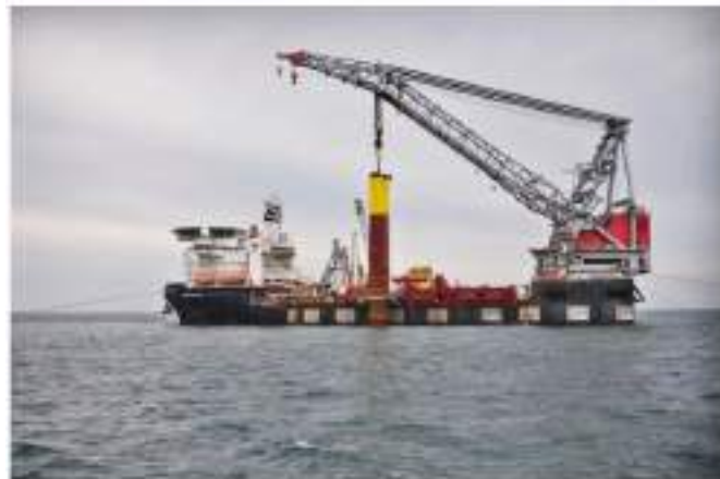
Vessel Seaway Strathmor on installation duty at Triton Knoll offshore wind farm. Image
