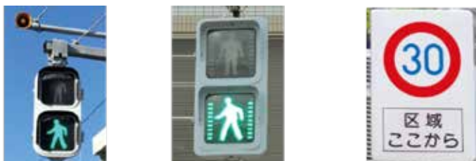
(Acoustic signal) (Lights with elapsed time display function for pedestrians) (Executing the maximum speed limit for which zone is set)
