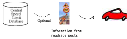
Figure 9. ISA based on roadside posts
