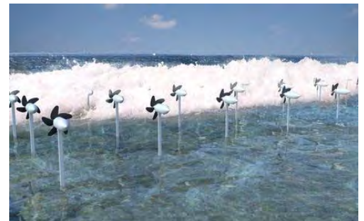
The inline small wave power generators generate electricity by utilizing a flow of an eddy generated from crumbling waves. (Imaged figure)
