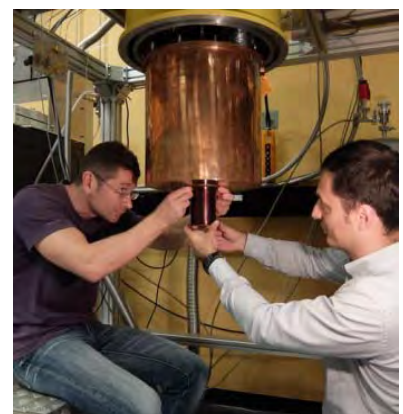
The super-conductive magnet used for the quantum experiment
