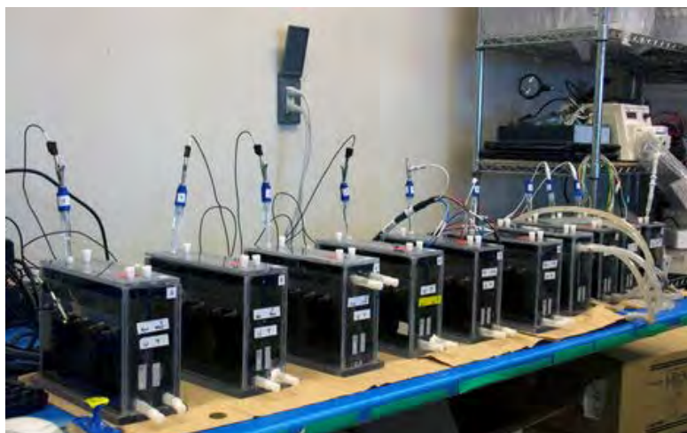
MFCs in the OIST Biological Systems Unit lab containing treated and untreated wastewater from the Okinawa Prefectural Livestock and Grassland Research Center.
