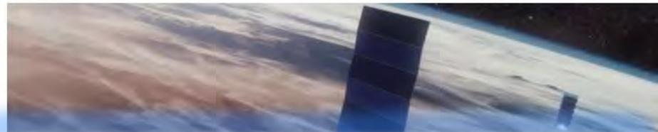
The 10 Starlink satellites launched to polar orbit Jan. 24 feature intersatellite links, a technology the company will expand to other satellites next year. Credit: SpaceX
