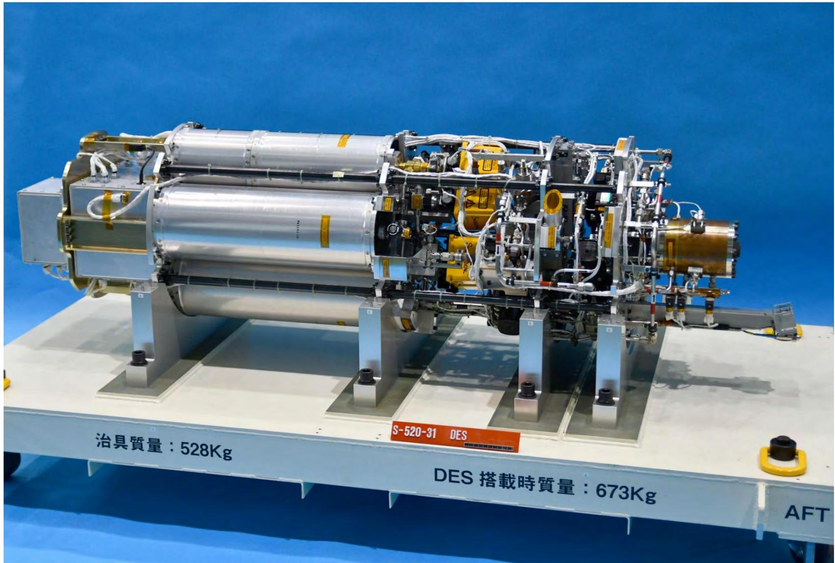
The Detonation Engine System Flight Model (DES-FM) of the S-520-31 sounding rocket was completed. It was confirmed that 530 N of thrust and  $1.5 \text{ m/s}^2$  of flight acceleration could be achieved by RDE operation.
