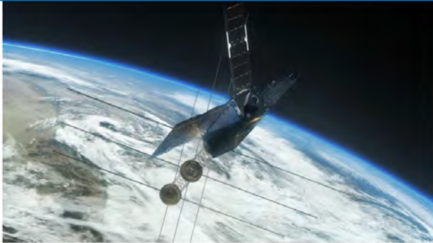
An OrbComm satellite provides AIS communications to shipping (source: メッセージ Saab)
