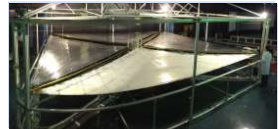
8 × 8m solar sail prototype by CAST
