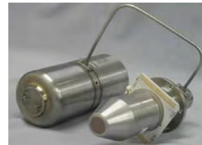
QDIP (Quantum Dot Infrared Photodetector)
