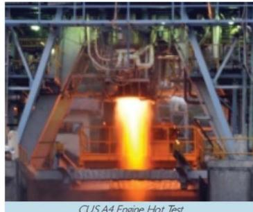
CUS(Cryogenic Upper Stage)燃焼試験
