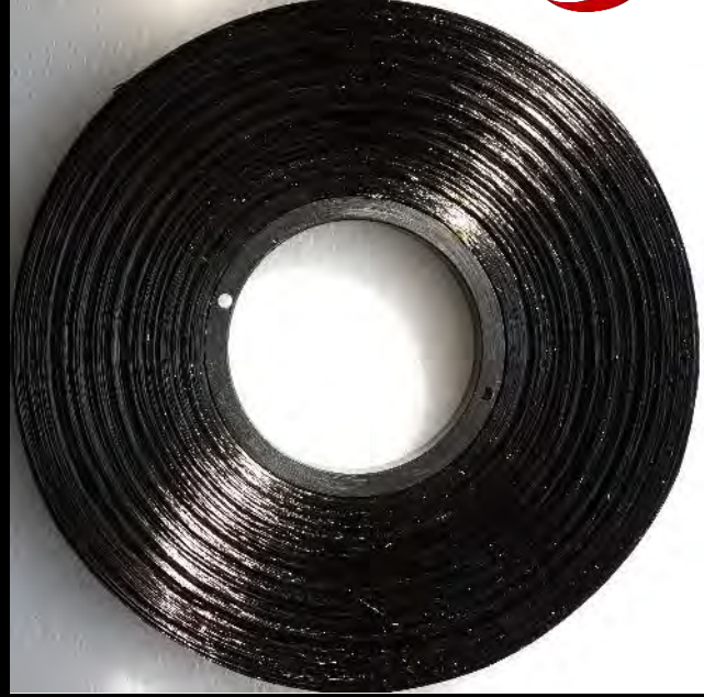
Polycarbonate Impregnated Pitch Carbon Fiber Tape* - LOX compatible -
